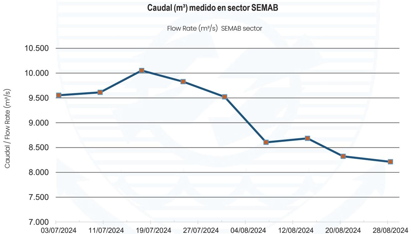
**Figura 39.** Evolución comportamiento caudal sección transversal km 8+500.
